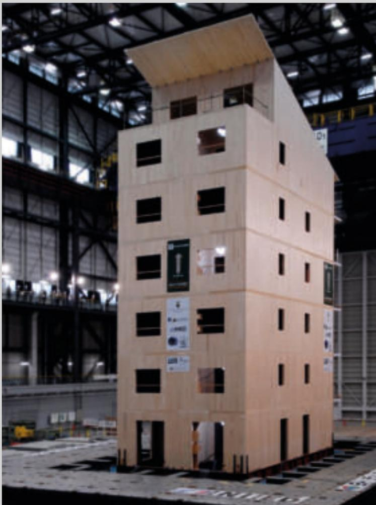
The XLAM panel (to be read: "cross-lam", where "X" indicates the orthogonal arrangement of the wooden elements that make up the panel) or CLT (Cross Laminated Timber) is an engineered timber product made of glued wooden layers staked crosswise. The XLAM panel is used as a load-bearing wall, floor, roof or as a partition element.
